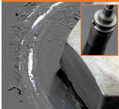
Standard socket – Heavy Damage
