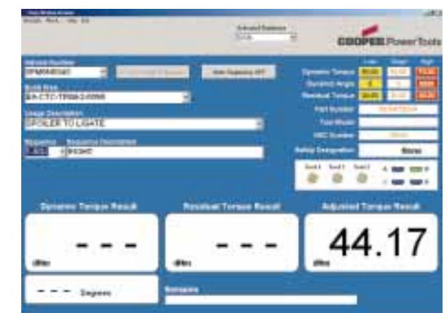
Adjusted Run Screen Adjusted Torque is NOK. Adjusted values are not evaluated for a high, OK or low. The background is always white.
