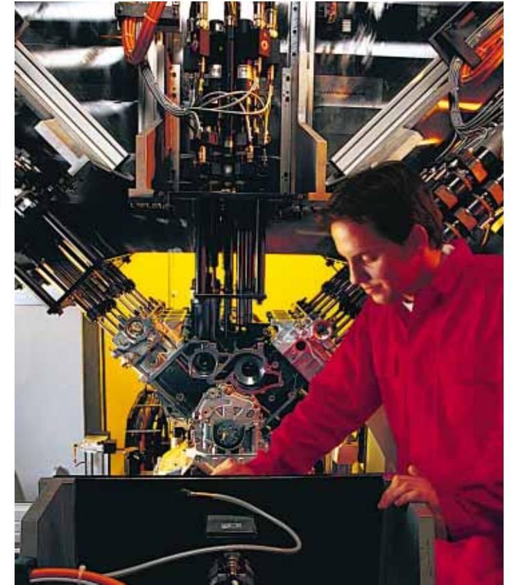
An automatic station on an engine assembly line uses two opposing electric power heads, each having 8 spindles, and a center power head of 6 spindles.
