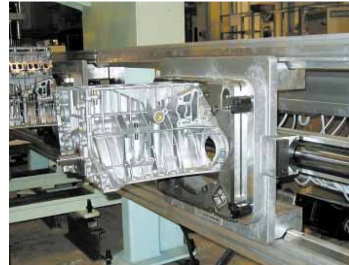
This GardoTrans installation shows a vertical system for floor level transport on the DaimlerChrysler Stuttgart 4 cylinder engine assembly line.
