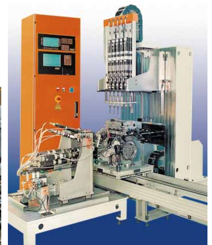
The GardoTrans 3 rail horizontal transport system shown at left is a typical engine assembly application.
