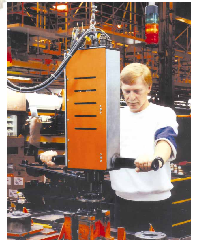
Repair bay operator is using a two spindle fixtured tool to fasten components of a wheel hub assembly.
