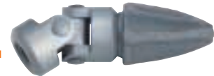
Drill Head with Universal Joint Range: 1-1/2 in. (38.1 mm) - 11 in. (279.4 mm) Deposit: 1/2 in. (12.7 mm) - thick-hard to medium
